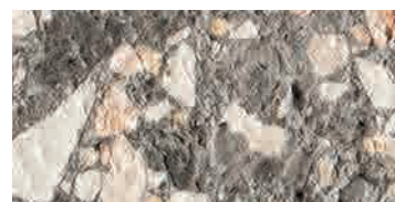
bocciardato / bush-hammered / gestockt
