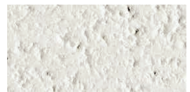
bocciardato / bush-hammered / gestockt
