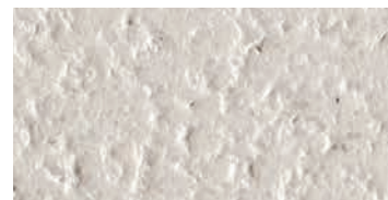
bocciardato / bush-hammered / gestockt
