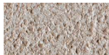
bocciardato / bush-hammered / gestockt
