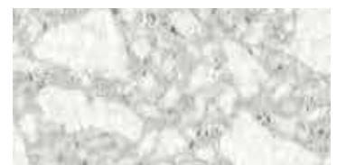
bocciardato / bush-hammered / gestockt
